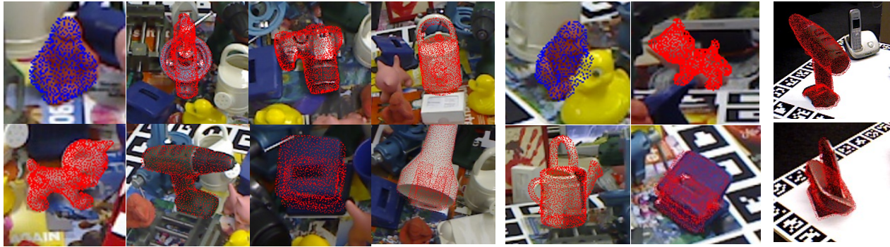
Fig. 9. Examples of object pose estimation results in LineMOD, Occlusion-LineMOD and HomebrewedDB. Object point cloud is transformed according to the predicted pose and then projected to the 2D image frame. Columns 1 to 4 depict the prediction in the LineMOD and Columns 5 to 6 show that in the Occlusion-LineMOD. Column 7 represents the pose prediction result in the HomebrewedDB.
