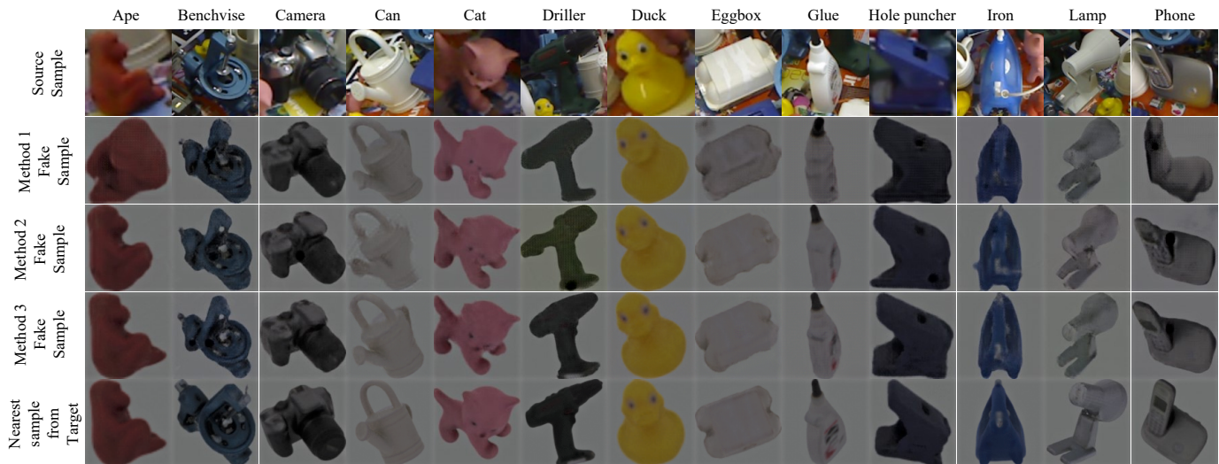
Fig. 7. The pixel-level real-to-sim domain adaptation results of the 13 objects in LineMOD. We exhibit the real-world (source domain) samples in the first row. The real-to-sim results generated by Method 1, 2, 3 are shown in the second row to the fourth row, respectively. The nearest neighbors of the generated fake samples in the simulation (target domain) are given in the fifth row.
