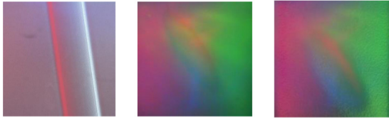
Fig. 9. Result of the modified simulator. The left is the original simulated GelSight image, the middle is the real DIGIT image, and the right is the simulated DIGIT image with our modified simulator.
